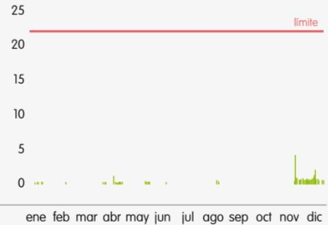
CASTEJÓN 3, EMISIONES HORARIAS  $\text{NO}_x$  ( $\text{mg}/\text{Nm}^3$ )
